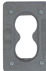
For standard and 3-pole, 2-wire grounding type duplex convenience receptacles; gasket included
